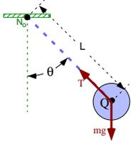
The moment of all forces on  $Q$  about  $N_o$  is calculated with the cross product of  $\vec{\mathbf{r}}^{Q/N_o}$  ( $Q$ 's position vector from  $N_o$ ) with  $\vec{\mathbf{F}}^Q$  (the resultant of all forces on  $Q$ ), as
