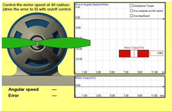
The point of this problem is to control  $\omega$  using an *on/off feedback control* for  $T_m$ .
