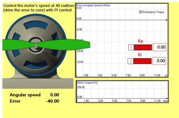
To answer each question with Working Model, click the **Reset** button (if necessary) and click and drag the sliders that control the feedback control constants  $k_p$  and  $k_i$  and try to keep the motor spinning at  $\omega = 40 \frac{\text{rad}}{\text{sec}}$ .
